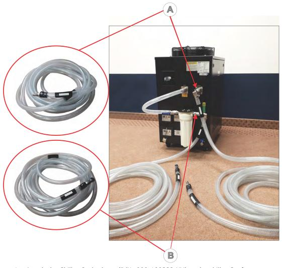
1. Attach the Chiller Outlet hose (P/N: 000-109323-XX) to the chiller **Outlet** port.
