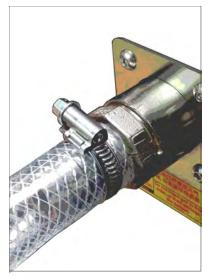
c) Tighten the worm gear clamp over both the hose and **Inlet** port as shown in the photograph until the hose bulges slightly on either side of the clamp.
