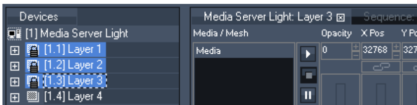
Figure 7a: The lock icon in front of the layer labels shows signifies a locked selection.
