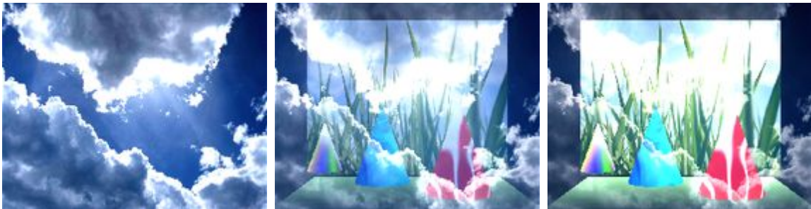
Adds the pixel values of the Target's texture with the ones of the Rendering. In case of values above 255 (in the case of RGB), white is displayed.
