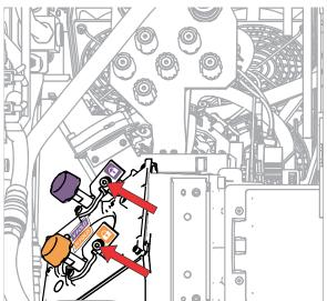
8. To make horizontal adjustments on the fold mirror, use the orange adjustment knob. To make vertical adjustments on the fold mirror, use the purple adjustment knob.
