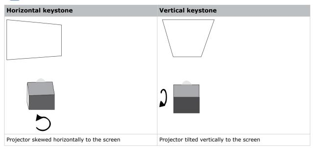
1. If the image suffers from slight keystone effect, it can be corrected with electronic cropping.
