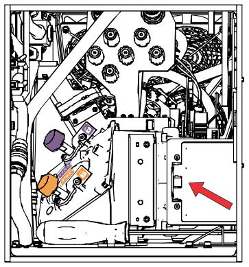
5. Loosen the lock screw for the Zoom and Focus paddles.
