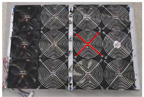
b) Attach the wire grille using four push rivets for each fan guard.
