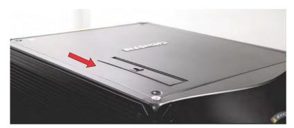
2. Secure the cover by tightening the four captive screws.
