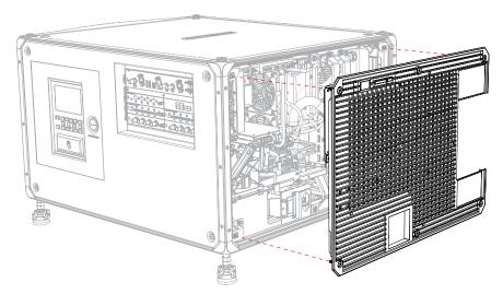
4. In the rear compartment at the panel mount, disconnect the DTSM harness (labeled Panel F) coming from the HKBB.
