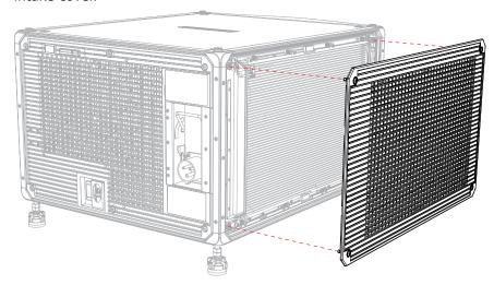
3. Loosen six captive screws to remove the rear cover.
