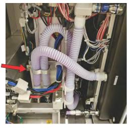
6. Place cloth wipes around the cooling hose connection points to capture any excess coolant that may drip upon disconnect.
