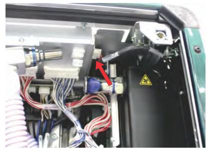
5. In the rear compartment, remove the hose bracket securing the coolant hoses by loosening the captive screw.
