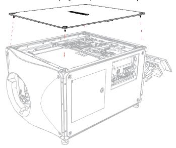
b) For CP4440-RGB and CP4450-RGB, loosen four captive screws securing the top-front cover.
