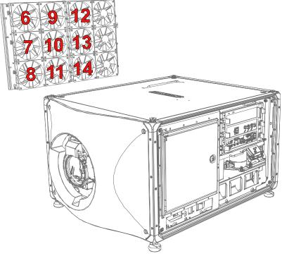
To confirm the correct fan positions, refer to the fan labeling on the projector.
