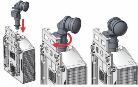
12. Place the lens with the lens connector aligned with the red notch position
