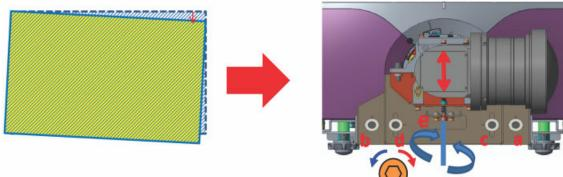
4. To fine-tune the image keystone-position, adjust the M6 screw "f" located on the top bracket with a 5 mm hex key.
