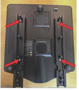
7. Secure the support base on the support beams with four M6 screws, lock washers, and washers with a 5 mm hex key.
