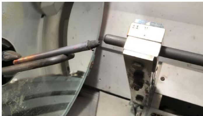
^ Pictured: A close view of two carbon rods used in carbon arc technology Source: Model, B. (2019, August 12) Shedding Some Light on Classic 35mm Film Projection. SilentFilmMusic.com/carbon-arc
