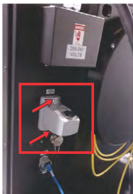
J33 terminal block 1 shown here with the location of the mounting screws indicated with the red arrows
