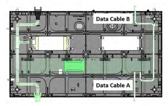
2. Connect an Ethernet cable from each Ethernet output port on the controller to the corresponding tile according to the connection diagram provided in the design package for your project.
