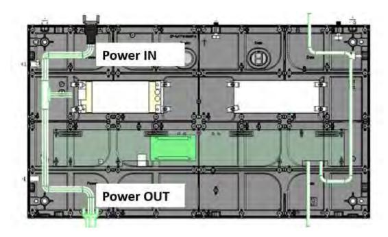
2. Connect the main power cable from the wall outlet to the top tile in each column of tiles in the array. Power cables must be connected top to bottom and only vertical connection within a column is possible.
