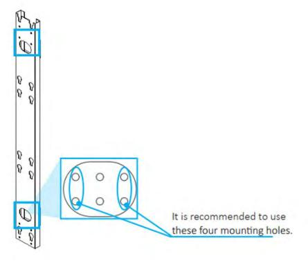
5. Use the mounting template to align the second vertical mounting pole.
