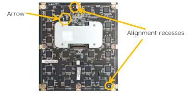
3. Set the LED module into place on the alignment recesses.
