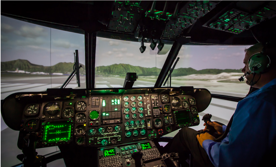
The cockpit of the CH-53E training simulator, featuring a 220 degree horizontal by 60 degree vertical image.
