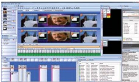
▲ Vista Advanced is a Windows-based software interface that makes it easy to configure and control the Spyder X20.
