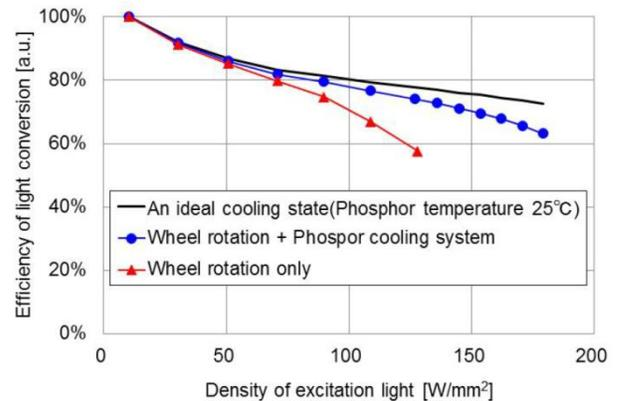
**Figure 1.** The dependence of laser-phosphor light-conversion efficiency on excitation density (from [2]).
