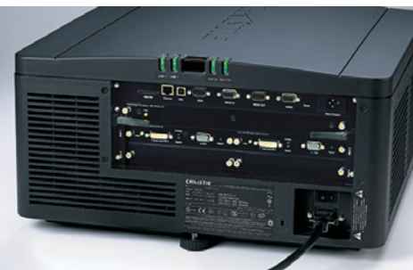
▲ Christie HoloStage standard configurations feature Christie Mirage M Series projectors that come standard with two high performance, full bandwidth 330 MHz dual link DVI-D inputs per projector. This feature enables the display of a frame-locked passive stereo source for high-performance active stereo at 120Hz without the need of a passive to active converter.
