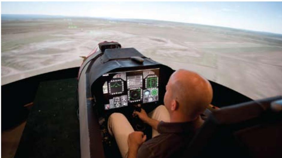
*Christie's seamless, blended screen with approximately 9 million pixels assists in the evaluation of various test bed/platform simulators for fidelity in simulation at Carleton University's ACE Lab*
