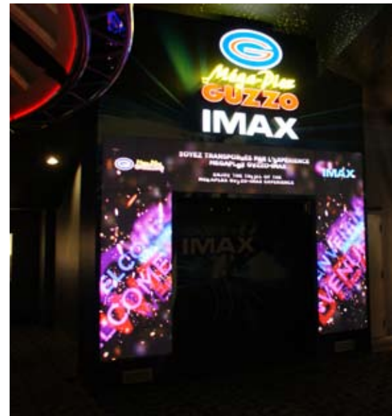
▲ The Christie MicroTiles get people to stop and look at the whole display.
