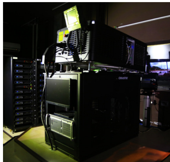
▲ Producing 45,000 lumens, the Christie CP42LH pure RGB laser projector illuminates Showtime Cinema's giant screen with brilliant color and detail.
