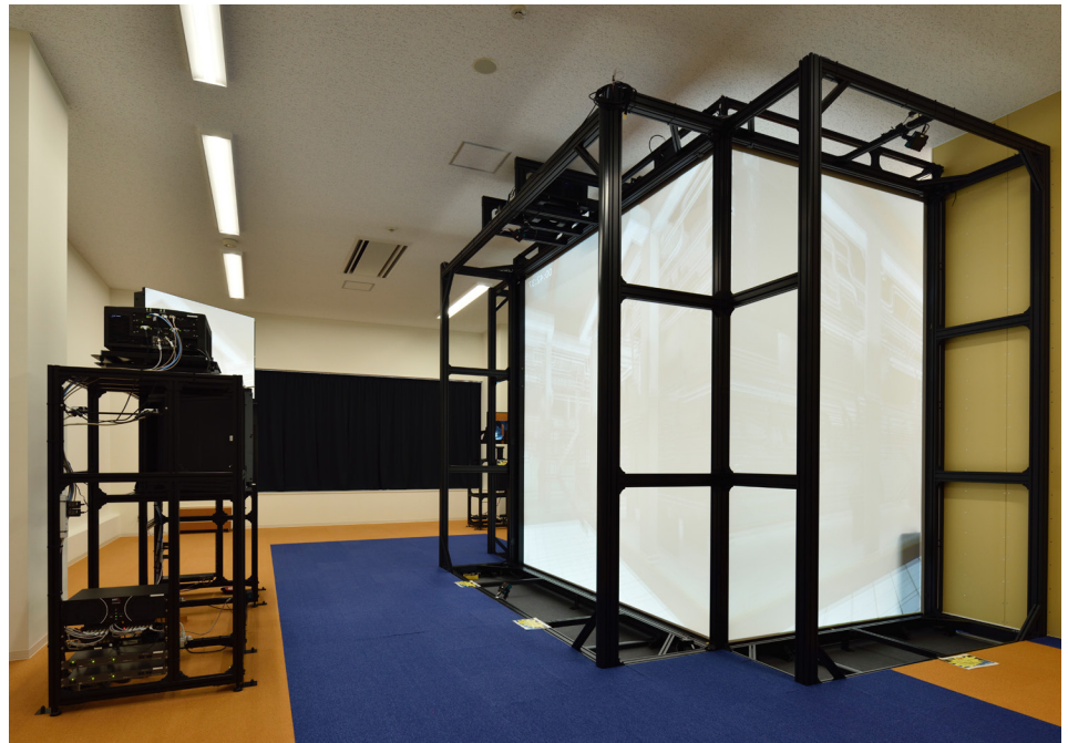
▲ Christie Mirage WU12K-M projectors display visuals of the Christie HoloStage system from the rear
