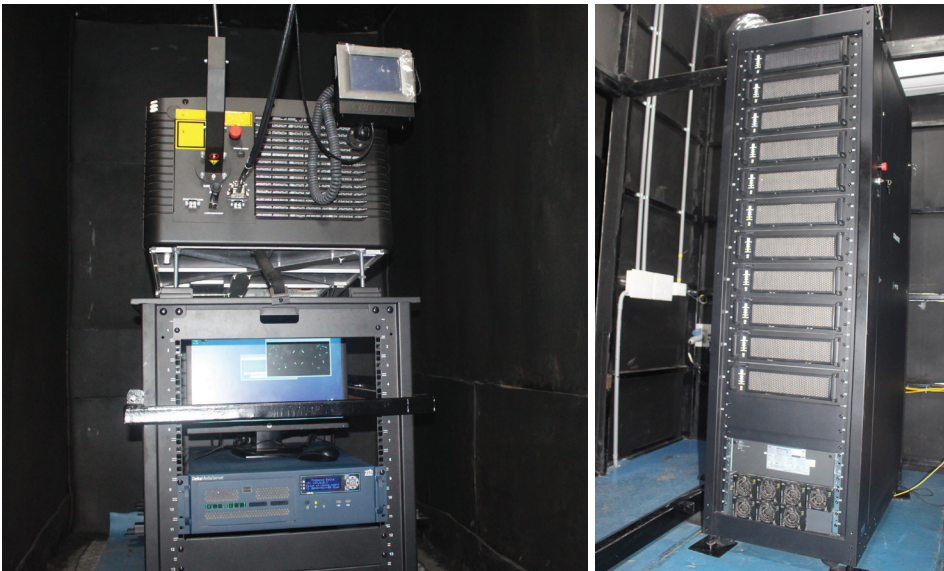
▲ The Christie D4KLH60 projector (left) and the laser rack fitted with laser modules (right) to deliver a brightness of 60,000 lumens on the parabolic screen
