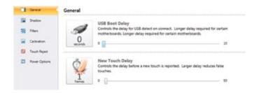
▲ The New Touch Delay feature controls the number of frames a touch object must exist before being reported as a valid touch event.
