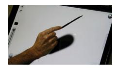
Optical systems featuring "Any Object" touch detection will register a touch from any solid object, such as the side of a palm.
