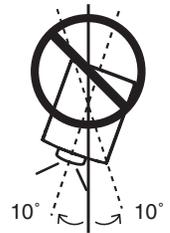
In downward projection, do not tilt the projector over 10 degrees right and left.
