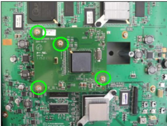
5. Install the dual processor warp board and secure with the 4 screws removed in step 4.
