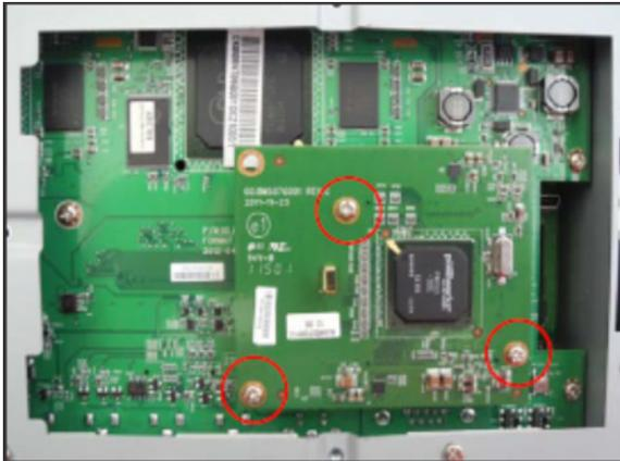
8. Install the dual processor warp board and secure with the 3 screws removed in step 7.
