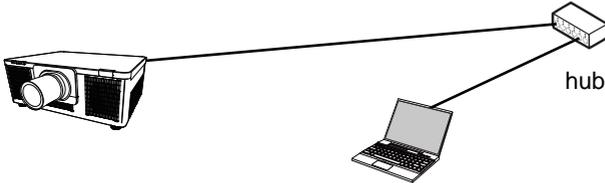
**■ Connection setup of wired LAN**
