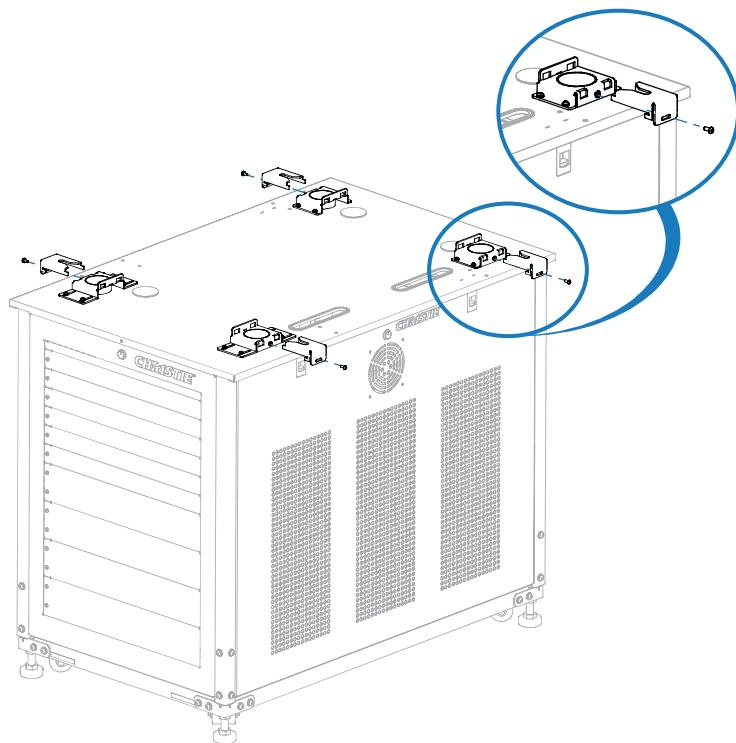
2. Install one screw in each of the four projector foot locks to secure them in position.
