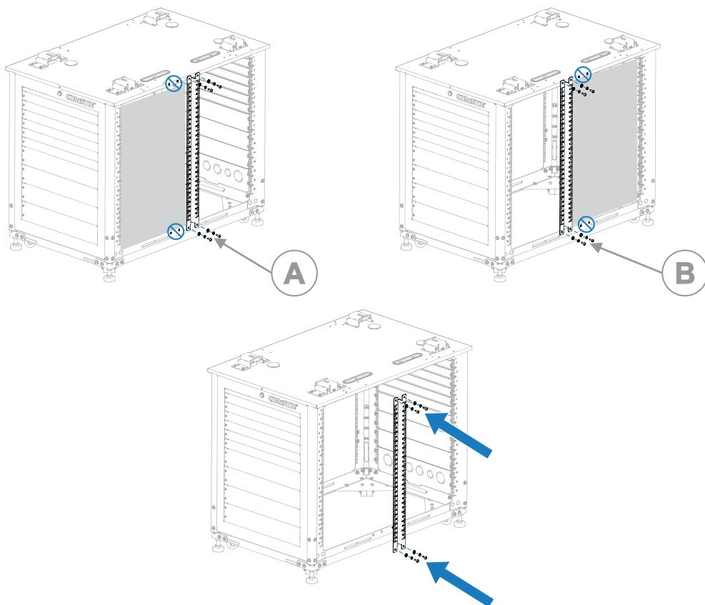
A Vertical support installed in the front mounting holes
