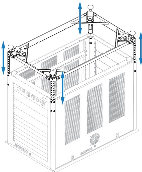
4. Make sure all four corners of the pedestal are adjusted to the same leg extension position.
