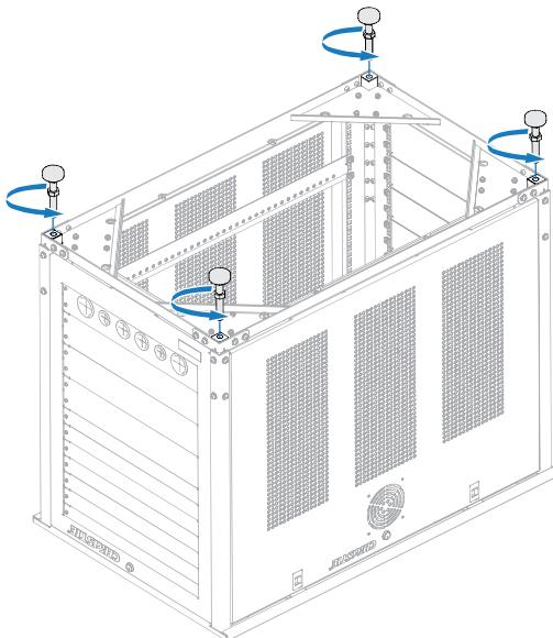
3. Thread one leveling foot into each of the four corners of the pedestal.
