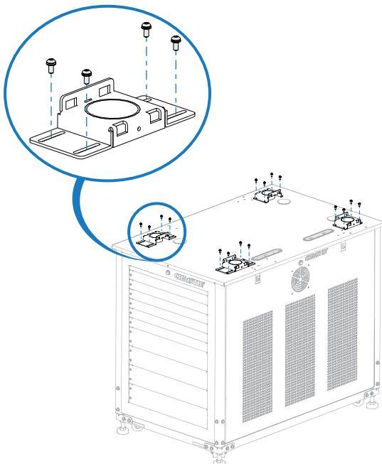
3. Loosely install the four screws in each of the four foot brackets.
