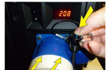
**⚠ WARNING** Do not attempt operation if the AC supply and cord is not within the specified ratings. On power down, wait 5 minutes for the fans to turn OFF before unplugging the projector. Always switch off the projector before unplugging the AC line cord.
