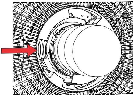
3. Turn the lens counterclockwise until the lens guides are aligned.
