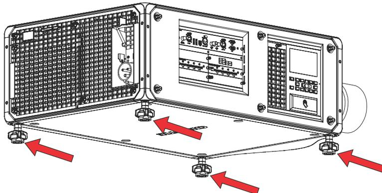
The projector feet are removable and can be moved to the top of the projector to run in an inverted orientation.
