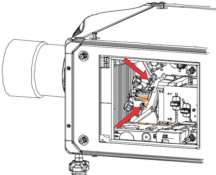
5. To make horizontal adjustments, use the orange knob labeled Horizontal.
