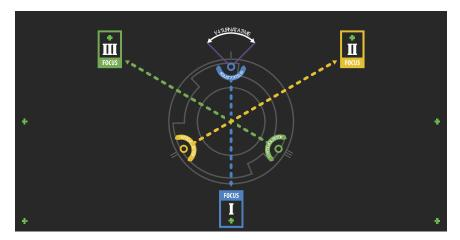
5. To focus the bottom boresight guide, adjust the blue boresight screw. Adjust the screw 1/4 turn. If you get to the end, further unlock the corresponding stabilization screw.
