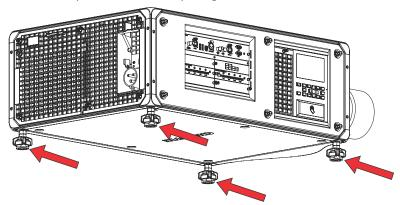
The projector feet are removable and can be moved to the top of the projector to run in an inverted orientation.
