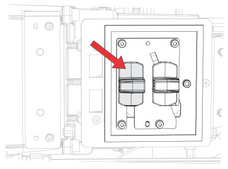
5. Adjust the focus using the Focus paddle. Always focus the center of the image first and then make sure no blurry edges exist.
