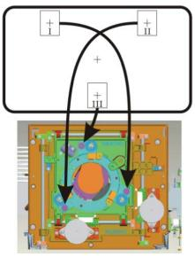
6. To fine tune the focus of cross-hair pattern I, adjust the appropriate capscrew (A on the rightside of the image below) until the cross-hair image is in focus with minimal flare.
