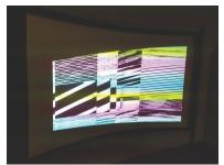
To recover from this issue, power cycle the projector with either the on-projector power buttons, or the projector power controls in the Twist software. After the projector is powered back on, the warp that is currently set on the projector should be modified so it does not induce warp limitation artifacts.
