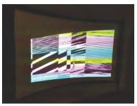
To recover from this issue, power cycle the projector with either the on-projector power buttons, or the projector power controls in the Twist software. After the projector is powered back on, the warp that is currently set on the projector should be modified so it does not induce warp limitation artifacts.
