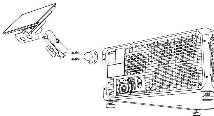
2. Install the ball arm onto the spacer.
