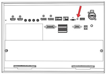
Before resetting the IP address to factory default, the light source turns on and remains on. The IP address is shown as described in *Determining the projector IP address* (on page 1).
