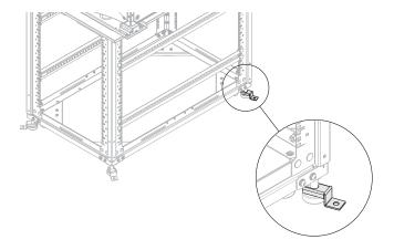
2. Secure the bracket to the floor.
