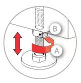
6. Once the required adjustment is made, tighten the lock nut against the bottom of the projector (B in the image in step 5).
