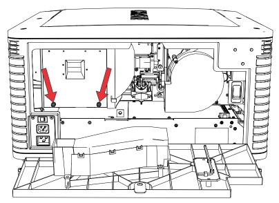
6. Loosen the cathode screw (D in the image below) with the 5 mm hex key attached to the lamp door.
