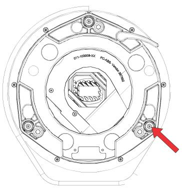
6. If the quality of the projected image has not improved, turn the right boresight screw 1/16 of a turn counter-clockwise.
