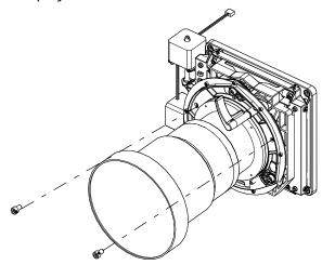
7. Lock the lens assembly in place by rotating the lens clamp downward.
