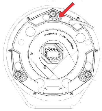
4. Turn the vertical screw 1/8 of a counter-clockwise turn.
