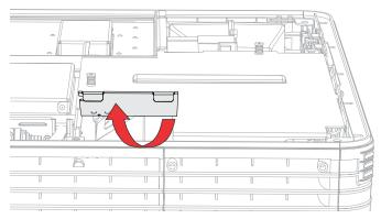
5. Loosen the two integrator rod screws.
