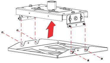
3. Tighten the four 5/16" nuts as shown in step 2.
