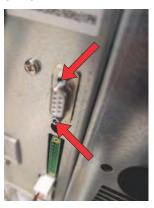
b) Install the two new standoffs provided in the chiller assembly kit (P/N: 152-161109-XX).
