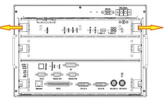
8. Pull the ICP outward out of the card cage and set it on a flat, stable surface.
