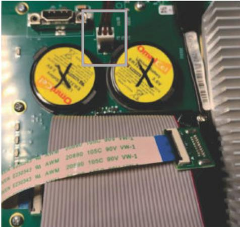
8. Replace the battery at the B1 location (shown in the image below).
