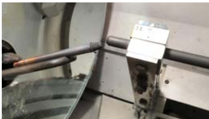
^ 图片:碳弧技术中所用两根碳棒近景,资料来源:Model, B. (2019, August 12) Shedding Some Light on Classic 35mm Film Projection SilentFilmMusic.com/carbon-arc
