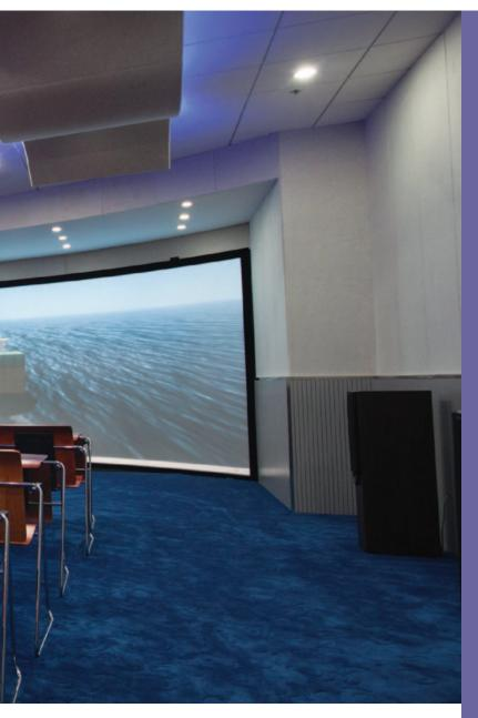
▲ JiaoTong University - Shanghai, China, features a 1x3 curved screen, 2.5 meters tall by 8 meters wide that displays a blended, seamless image with a 90-degree field of view.
