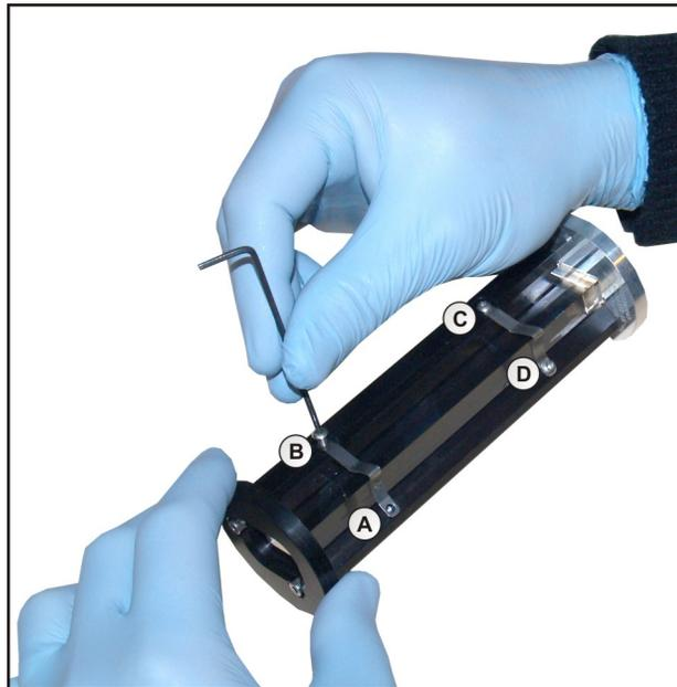
**Figure 4 Remove Existing Springs**
