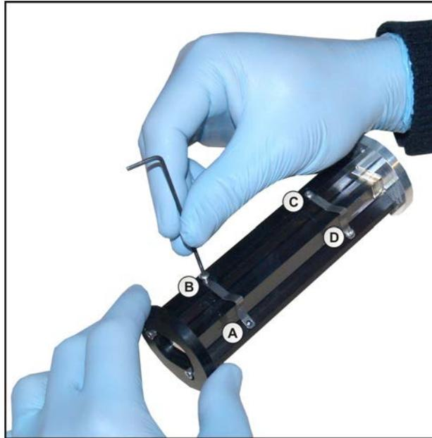
**Figure 4 Remove Existing Springs**
