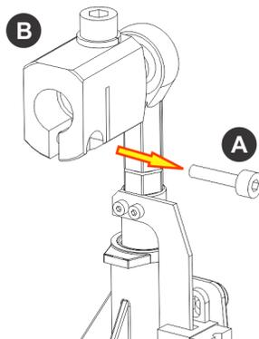
3. Insert and tighten the cathode screw into the opposite side of the cathode clamp.
