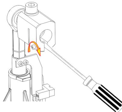
6. Remove the cathode screw and reinstall it in its original location.
