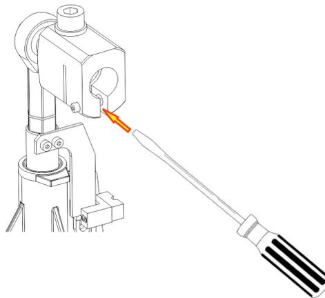
5. Hold the screwdriver in position and tighten the cathode screw against the screwdriver with a 1/8" Allen key until the cathode clamp widens enough to allow the installation of a CDXL lamp.
