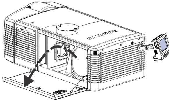
5. Undo the three clips on the cathode lamp duct and remove the duct.
