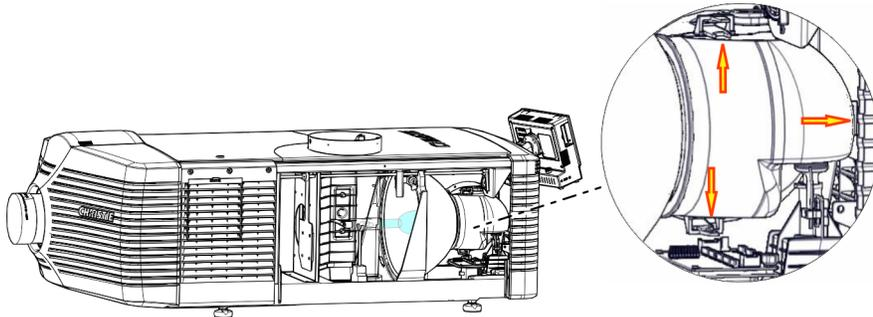
6. Loosen the cathode screw on the cathode clamp.
