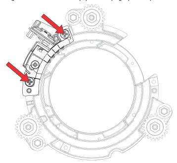
3. Tighten the middle screw (C) on the pogo pin adapter.
