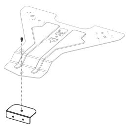
8. For the 630-GS and 635-GS models only, install the rubber spacer provided in the installation kit on top of the default rubber spacer on the lens support bracket.
