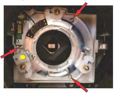
4. Install the connector you disconnected in step 1 on the new boresight adapter plate.
