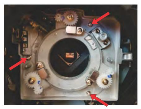
• Remove the four securing the boresight adatpter plate 2 (LSM2).
