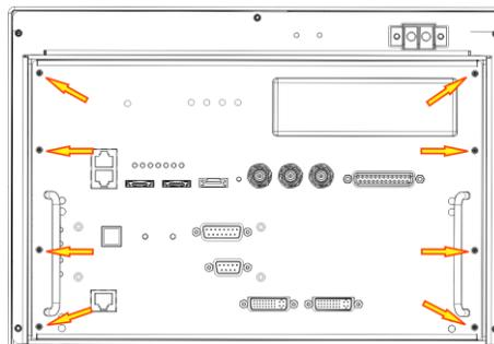
5. Remove the card cage faceplate by the handles and set it on a stable surface.
