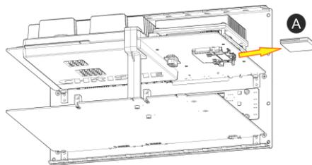
3. Slide the new CF card into the housing and then push the retaining clip down.
