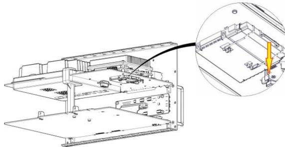
2. Pull the CF card (A) out of the housing and discard it following your local regulations for electronic waste disposal.
